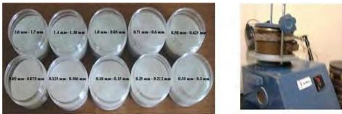
**Figure 2:** (a) Glass beads of different sizes used in the determination of Apparent Opening Size (AOS) of a geotextile (b) Sieving apparatus mounted on sieve shaker
